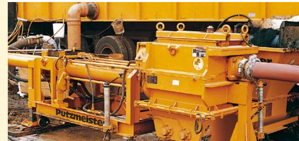
Mobile dewatering and pumping station
