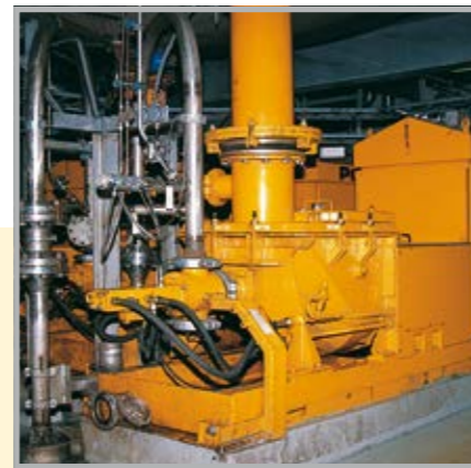
KOS 1070 coal sludge injection pump
