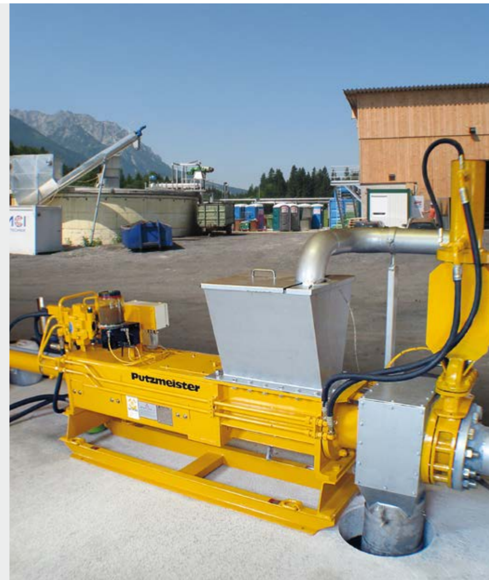
An EKO 1060 PP in a biomethanisation plant (Kössen, Austria) for unwrapping and transporting foods past expiry date
