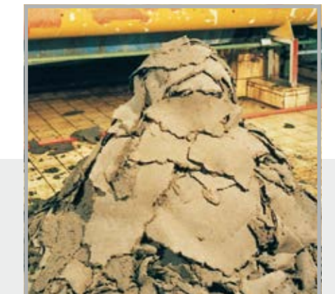
Sewage sludge dewatered by a chamber filter press: Solids content > 35 % DS
