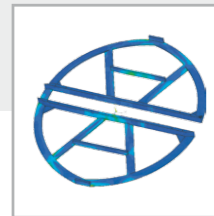
Finite element analysis for the sliding frame
