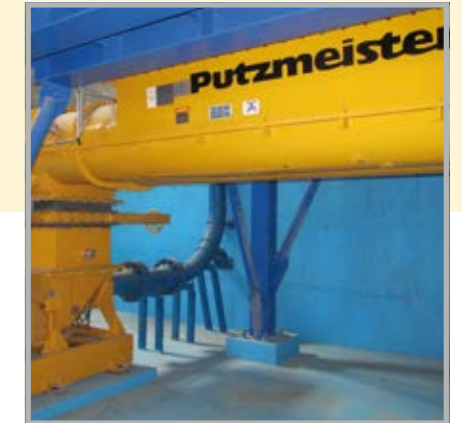
Twin-screw conveyor SHS 3262 SH
