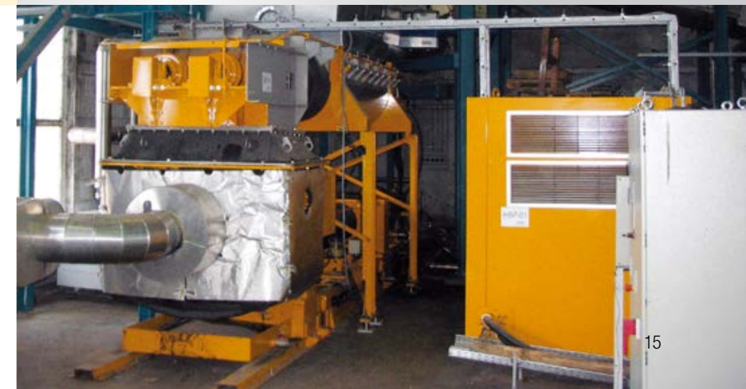
KOS 25100 with hydraulic power pack and twin-screw feeding device, transporting biomass to the fermentation tank
